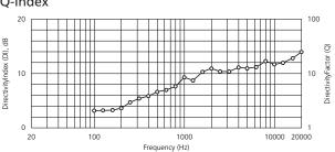
All measurements under free field conditions. Frequency diagrams 1/6 octave averaged, radiation and polar pattern 1/3 octave averaged. The manufacturer reserves the right to make product alterations to improve product quality without prior notice. Errors excepted.
