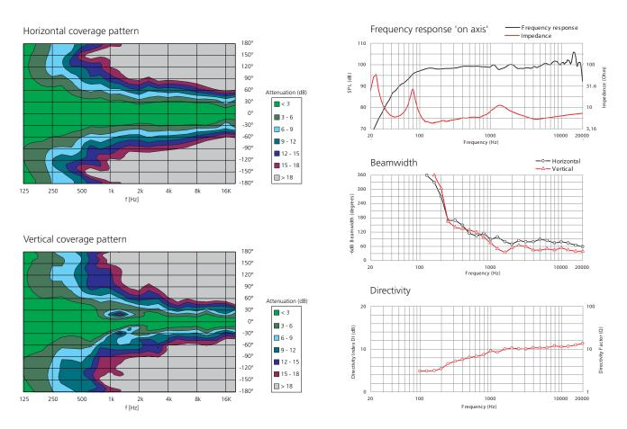
All measurements under free field conditions. Frequency patterns 1/6 octave averaged. Coverage and polar pattern 1/3 octave averaged. The manufacturer reserves the right to make product alterations to improve product quality without prior notice. Errors excepted.
