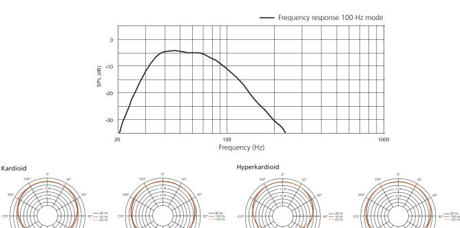
All measurements under free field conditions. Frequency patterns 1/6 octave averaged. Coverage and polar pattern 1/3 octave averaged. The manufacturer reserves the right to make product alterations to improve product quality without prior notice. Errors excepted. Attenuation factor depends on setting and configuration.
