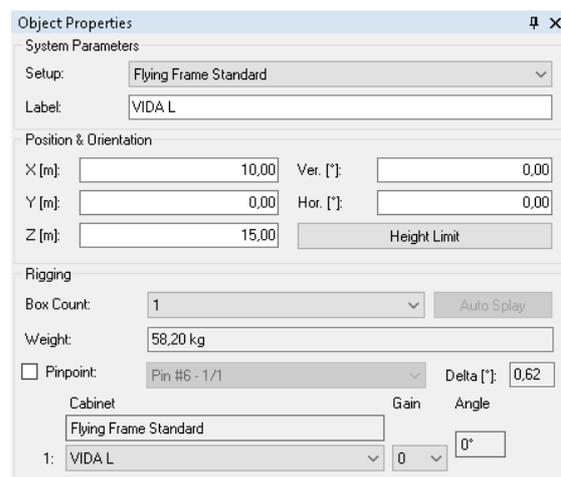
The *Gain* of each module in the array can be adjusted but the angle between the several modules needs to stay the same. Because of that the *Auto Splay*-Function (used in *Sequenza 5* and *-10* Setups) has got no real effect when setting up a VIDA simulation.
