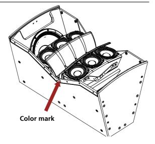
8. Replace the previously removed screws [B] to fasten the K&F VariQ unit.
