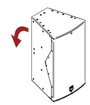
2. Remove the grille screws [A], then remove the grille.
